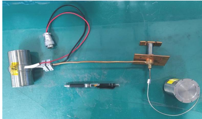
Figure 1. Experimental pulse tube cryocooler (PTC).
